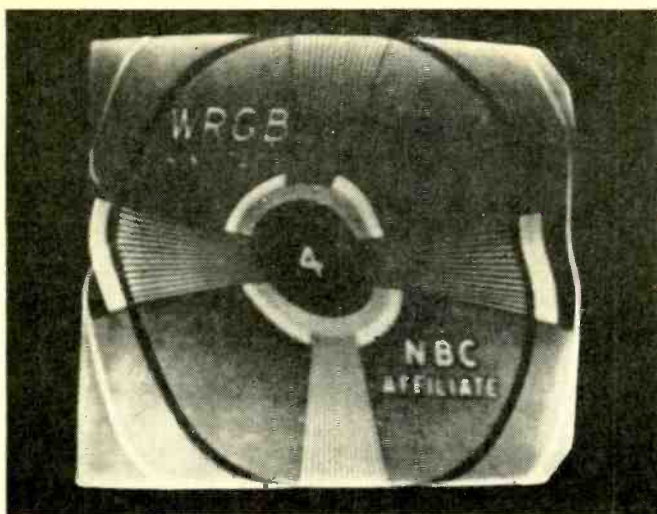
Fig. 2—Sixty-cycle hum modulation.
