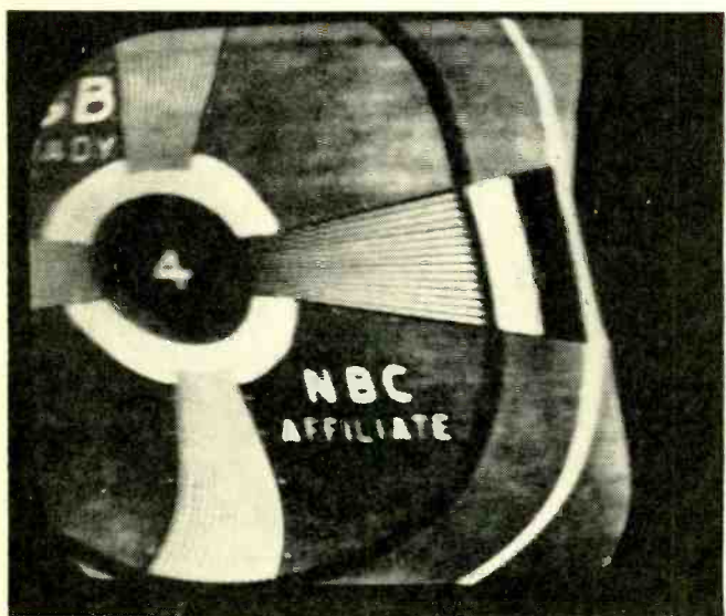
Fig. 3—Horizontal bend due to cathode-heater short in sync amplifier.
